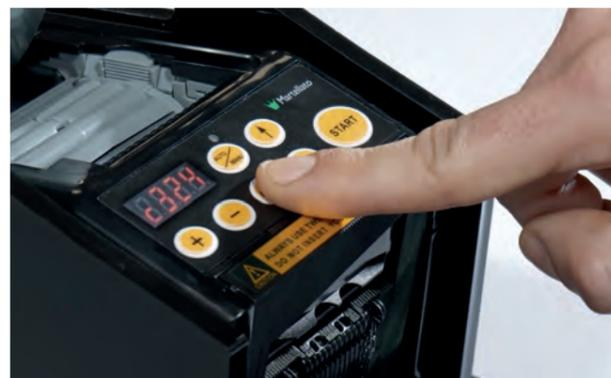
Press Select to select one of the 6 preset cutting lengths. You can change the cutting lengths using the +/- keys. Press Select again to reset the desired number of strips, from 1 to 999. Press Start to start cutting.
